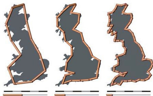
The coastline paradox: a map of Great Britain’s coast using progressively shorter increments of measurement
