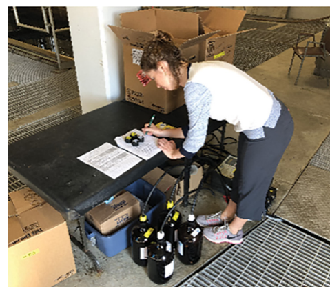
Lisa Erdle sampling the water at the waste water treatment plant in Parry Sound to get base level readings before the filters are installed.
